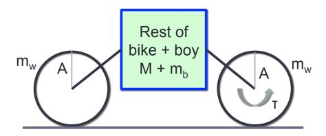
The bike itself is taken to have mass  $m_b$  plus the mass of its two wheels, each providing  $m_w$ , plus M for the boy. The wheels have radius A and the moment of inertia of a ring  $I = m_w A^2$ .
