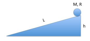
A hollow cylinder, a solid cylinder and a sphere roll down a hill. They all have mass M = 10.0 kg and radius R = 1.00 m, and start at rest a distance L = 10.0 m up the hill, corresponding to a difference in vertical height between top and bottom of h = 1.00 m. The moment of inertia of a hollow cylinder is  $MR^2$ , of a solid cylinder  $MR^2/2$ , and of a sphere  $2/5 \times MR^2$ . There is gravity g = 9.80 m/s<sup>2</sup>.
