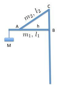
A lamp post consists of a vertical pole, a horizontal bar of mass  $m_1$  and length  $l_1$  attached to it at a point B, and a diagonal bar of mass  $m_2$  and length  $l_2$  attached to it at a point C, as shown in the Figure. The horizontal bar is attached to the diagonal one at a point A, a distance h from point B. At the end of the horizontal bar, a lamp of mass M has been attached, hanging straight down. The system is in static equilibrium.
