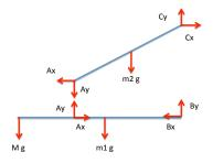
b) Write down the torque equations, so that both horizontal bar and diagonal bar do not rotate. For each of the two bars, use an axis at A.
