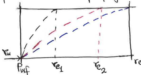
iii) It will take some time, from a few months, to a couple of years, for ~~the~~ <sup>during transient</sup> ~~5~~ pressure waves to develop from the reservoir, to ~~the~~ reservoir boundaries. At this point, the pressure at every point in the reservoir will be constant, if we have strong pressure support from an aquifer. The flow regime now is "Steady-State".
