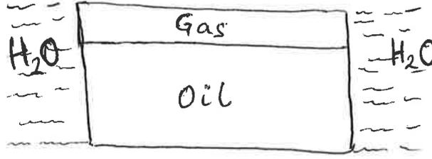
The reservoir has a gas-cap and water at the edge of the reservoir boundaries.
