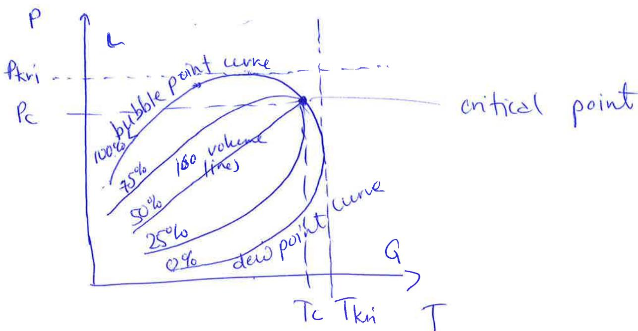
Two phase envelope: given by bubble point curve and dew point curve.
