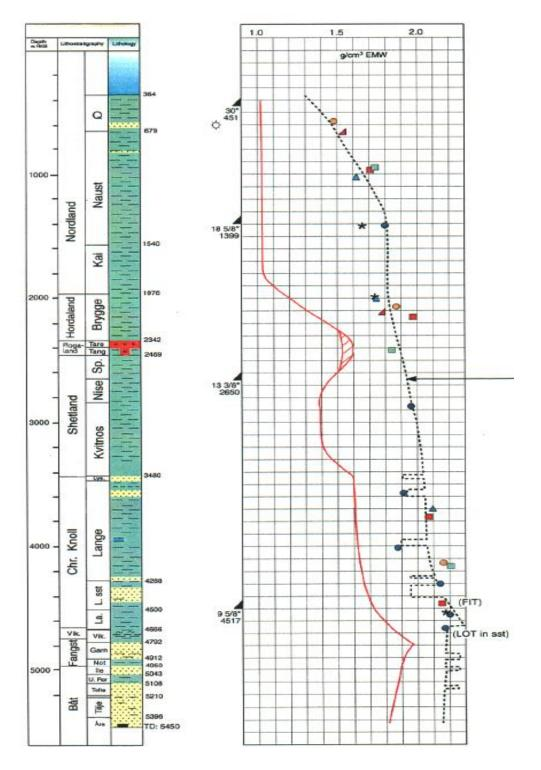
2) Explain shortly what a kick tolerance is and how it affects the casing shoe depth selection. Also explain why they chose to set the 9 5/8" shoe below the weak fracture pressure zone.
