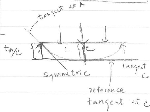
using moment area method, considering half of the beam (symmetric).
