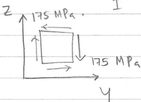
$$\begin{aligned}\text{Total shear stress at A} &= 169 + 6.04 \\ &= \underline{\underline{175 \text{ MPa}}}\end{aligned}$$
