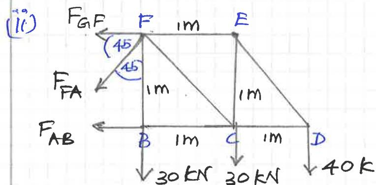
Axial forces of members using method of section.
