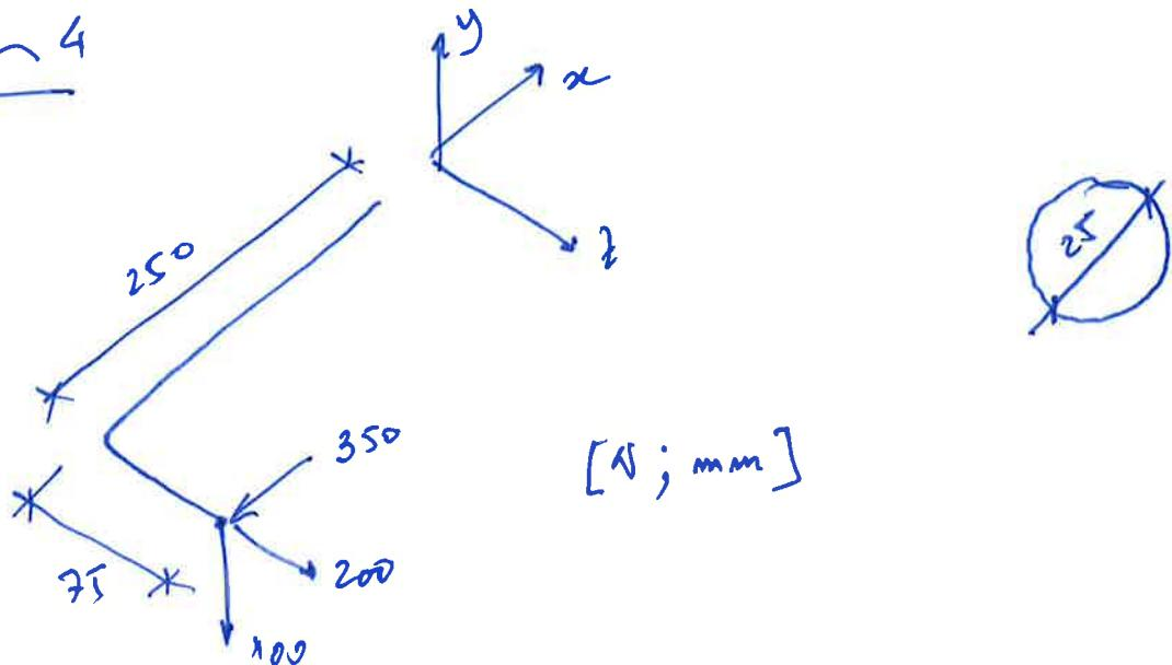
① Determine the internal forces at section A-B using Free body diagram and the 6 equations of equilibrium.
