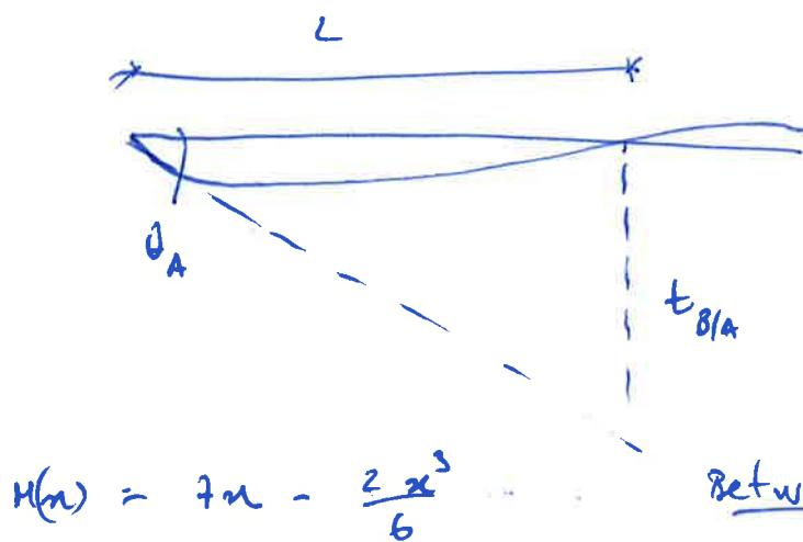
$$Q_A \times L = t_{B/A} = \frac{1}{EI} \int_A^B M(x) x \, dx$$
