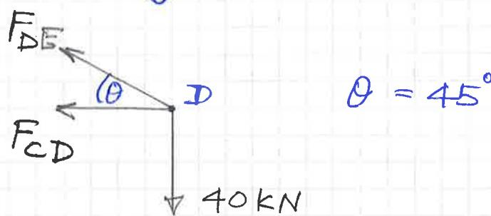
Using method of joints, considering equilibrium of joint D,
