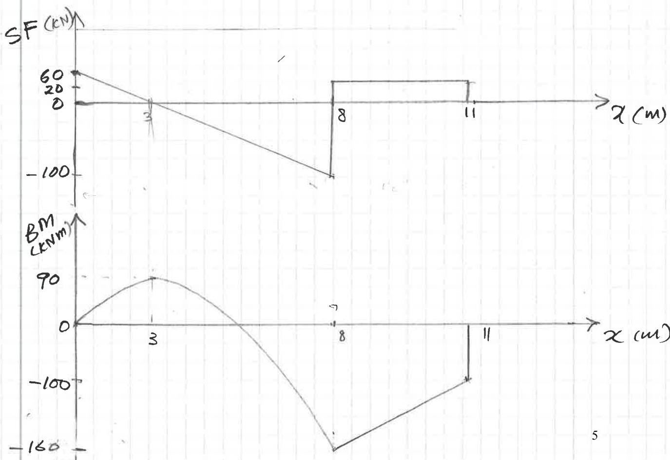
Shear force and bending moment diagram
