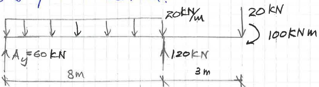
slope  $\frac{dV}{dx} = -w(x)$   $\frac{dM}{dx} = V(x)$
