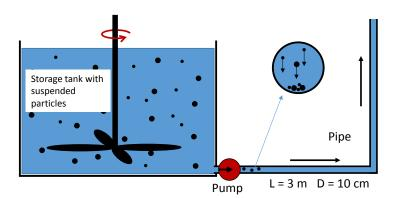
The particle concentration (by volume) in the tank is 5%. The particle diameter  $d_p$  ranges from 100  $\mu$ m (micrometer) to 1500  $\mu$ m. The particle density is 2.6 g/cm3.
