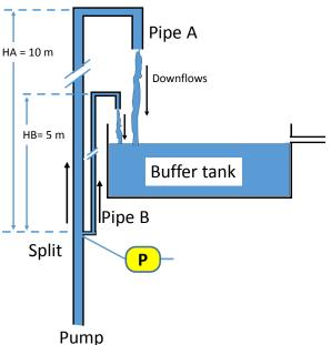
two pipes from the start position start, until finally stabilized? What is the pressure P at the split just when liquid starts to flow out of pipe B?
