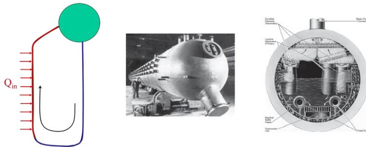
Figure 23: Schematic figure of natural circulation, and picture of a drum
