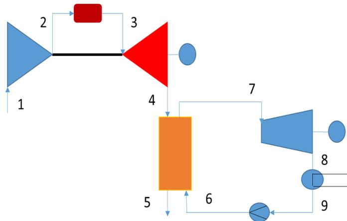
Figure 49: Schematic simple combined cycle
