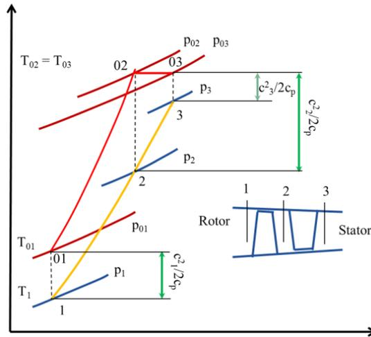
Figure 33: Changes in flow properties over the compressor stage illustrated in a TS-diagram
