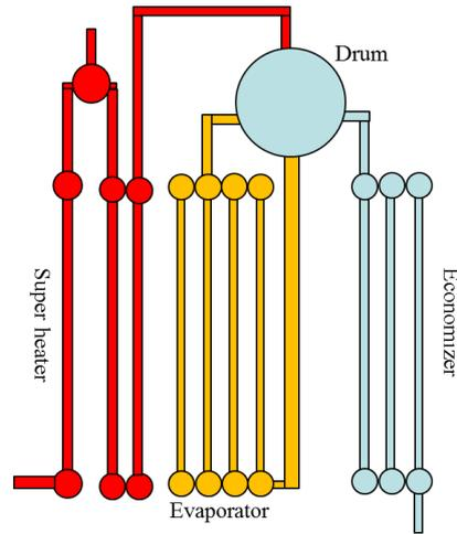
Figure 50: Heat transfer surfaces in single pressure HRSG
