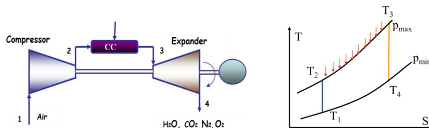
Figure 28: Ideal gas turbine cycle with 100% compressor and expander efficiency ( $\Delta S=0$ )
