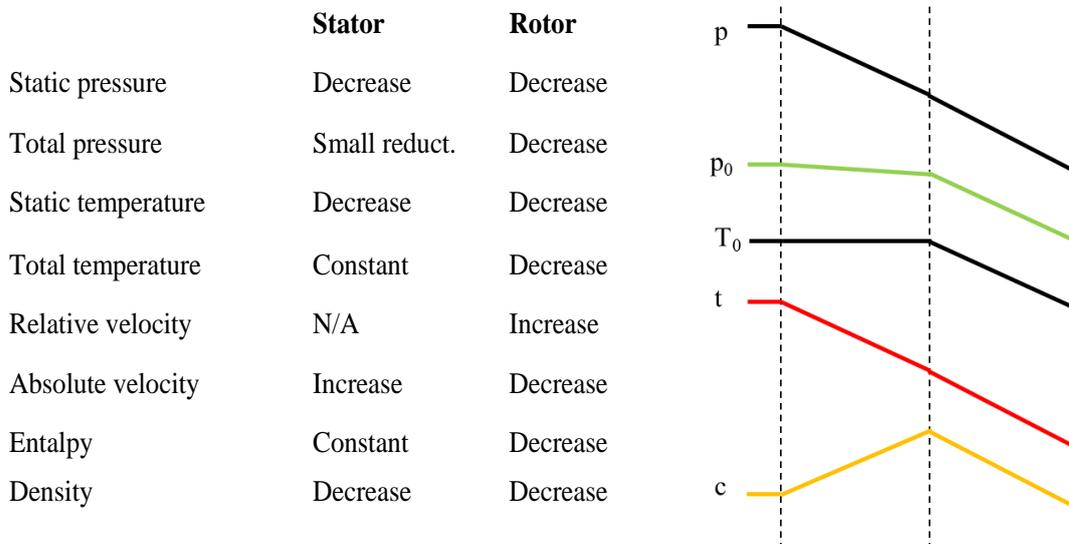
Figure 36: Change of properties of the working fluid
