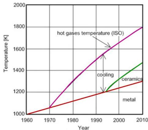
Figure 39: Development of TIT and impact of various technologies
