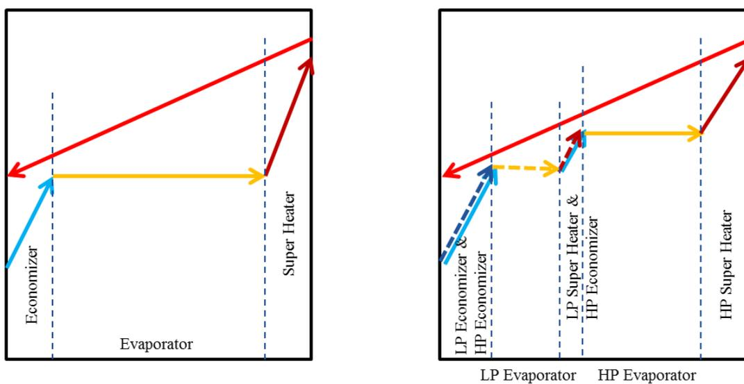
Figure 52: Schematic heat transfer for one and two pressure level HRSG in TQ-diagram
