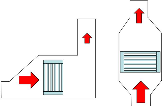
Figure 53: Schematic illustration of horizontal (left) and vertical (right) HRSG
