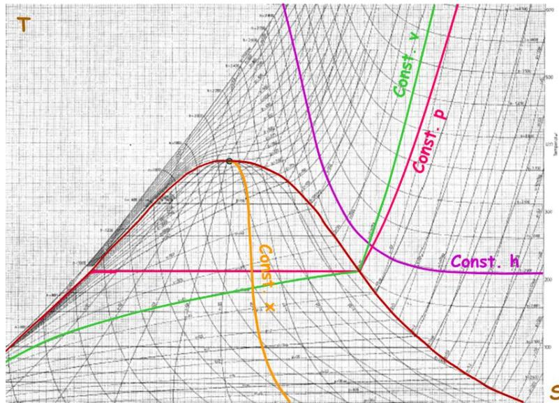
Figure 8: TS-diagram for water-steam, with highlighted constant pressure, enthalpy, specific volume and steam quality or dryness factor
