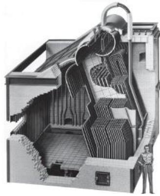
Figure 22: Internally fired boiler, 1933
