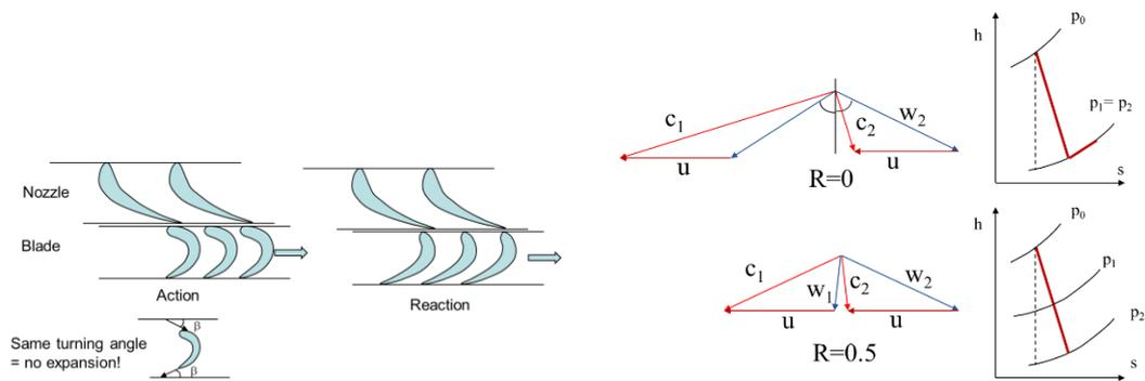
Figure 19A: Action and reaction blading. No expansion (pressure change) over blades of action stage only turning the flow
