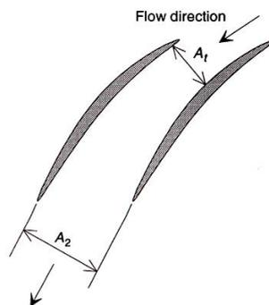
Figure 31: Outlet area of the blade passage is larger than the inlet area, resulting in velocity reduction
