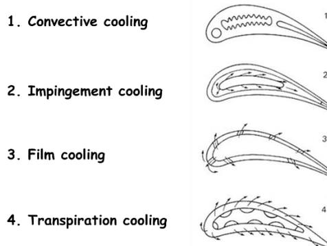
Figure 42: material cooling techniques
