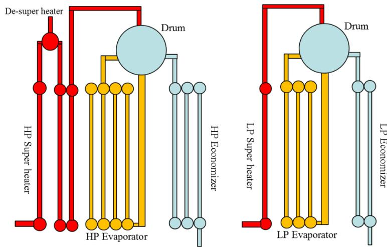
Figure 51: Heat transfer surfaces in two pressure HRSG
