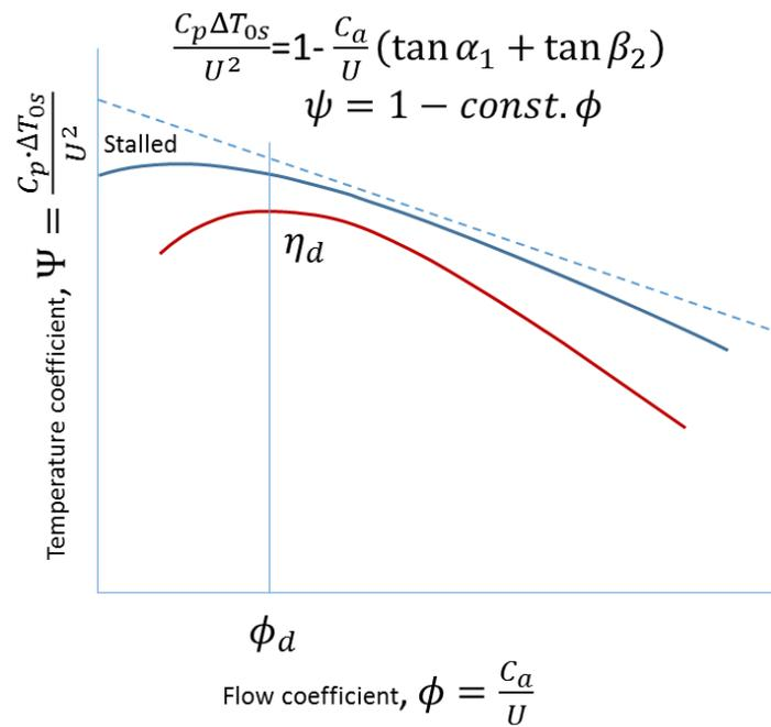
Figure 34: Compressor stability
