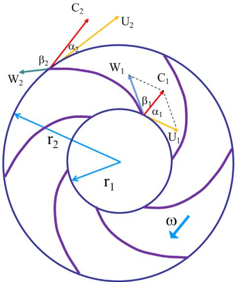
Figure 17: Velocity vectors at inlet and outlet of a centrifugal pump
