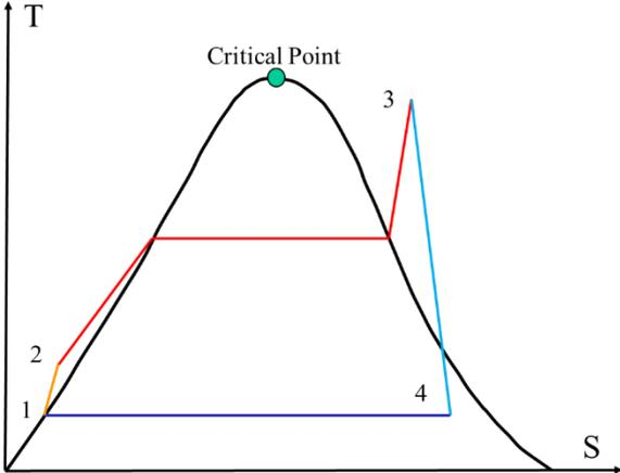
Figure 7: Impact of turbine and pump efficiencies on expansion and compression lines (increasing entropy between inlet and outlet of the component)
