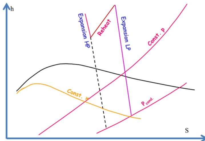
Figure 15: Expansion in the turbine and steam quality at the outlet
