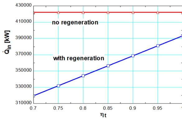
The effect of turbine efficiency on heat input to the cycle in two cases
