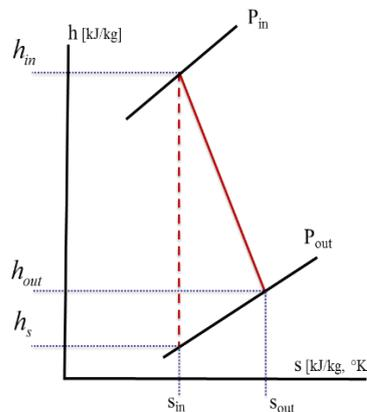
Figure 10: Expansion in the turbine, between inlet and outlet pressure
