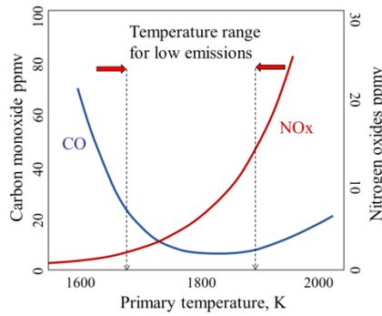
Figure 45: Emissions formation as function of temperature
