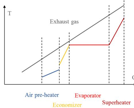
Figure 26: Heat transfer in various parts of the boiler, including air pre-heater
