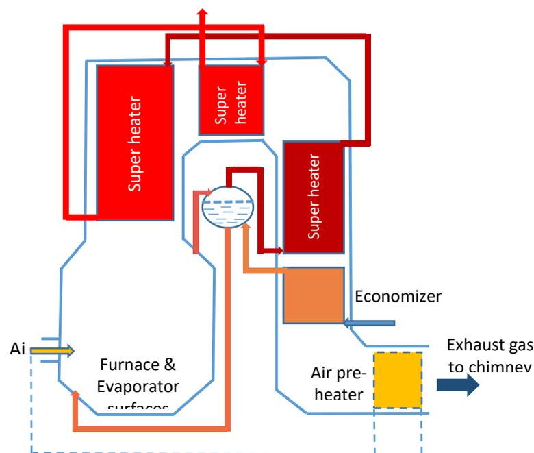
Figure 21: Schematic drawing of a boiler with heat transfer surfaces
