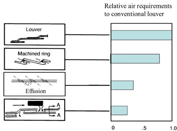
Figure 48: Relative cooling air for various cooling concepts
