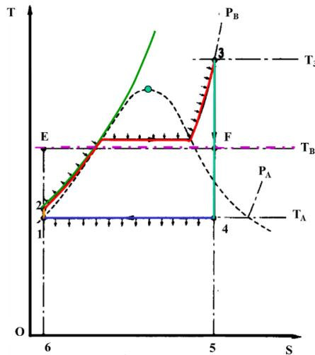
Figure 4: Steam cycle components in a TS-diagram
