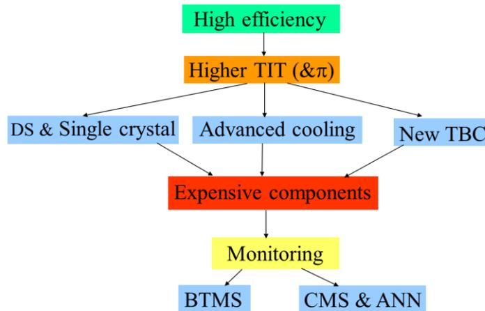
Figure 40: Reaching high efficiency and safe operation require optimized combination of TIT and PR, material cooling and monitoring techniques
