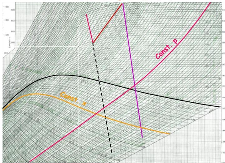
Figure 9: hS-diagram for water-steam, with highlighted constant pressure, and steam quality or dryness factor as well as expansion lines for single (dotted) and reheat turbine
