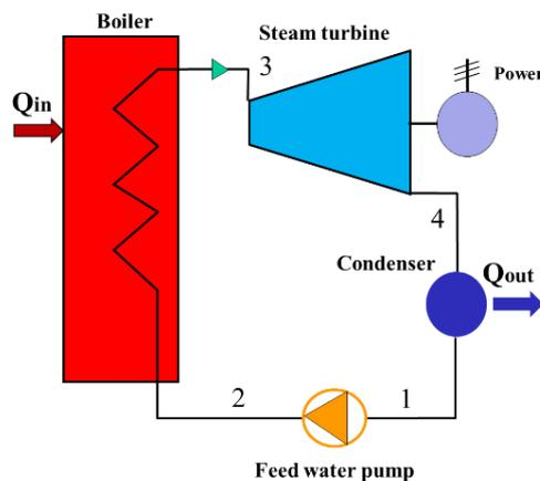
Figure 2: Schematic of a simple steam cycle
