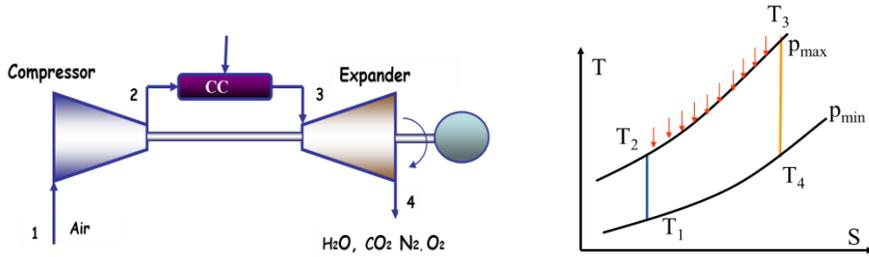
Figure 29: Ideal gas turbine cycle with 100% compressor and expander efficiency ( $\Delta S=0$ )
