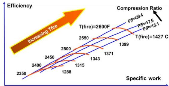
Figure 38: optimized combination of TIT and PR for combined cycle
