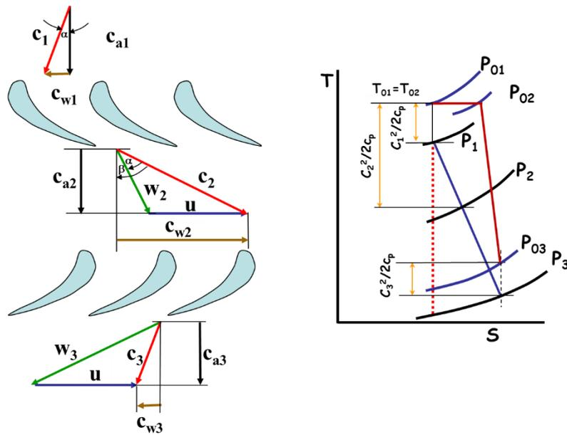
Figure 37: Expansion in TS diagram
