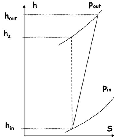
Figure 11: compression in the pump, between inlet and outlet pressure
