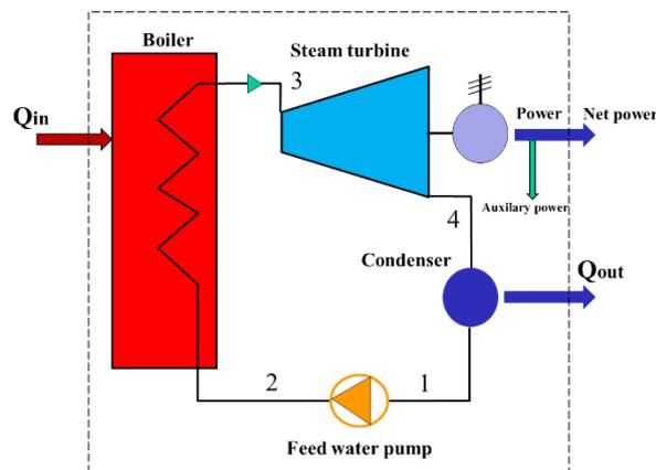
Figure 12: Energy exchange over the system boundary, covering only the steam side
