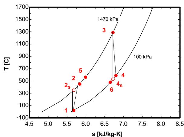
T-s diagram for gas turbine with regeneration
