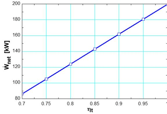
The effect of turbine efficiency on net work out in two cases
