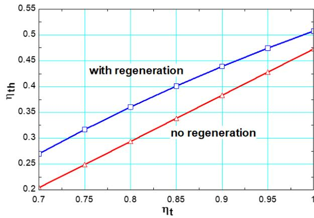
The effect of turbine efficiency on thermal efficiency of the cycle in two cases
