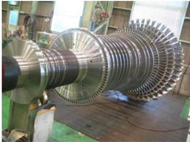
Figure 20: A typical steam turbine rotor
