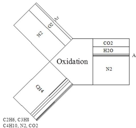
Figure 44: Combustion process
