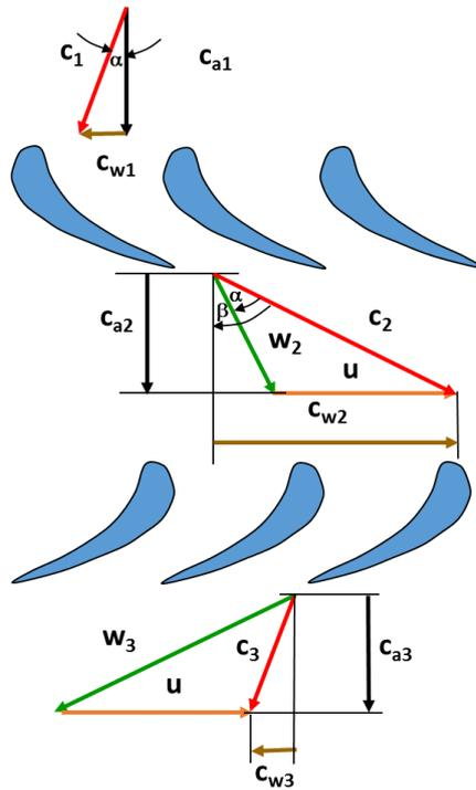
Figure 35: Velocity triangles for the turbine stage
