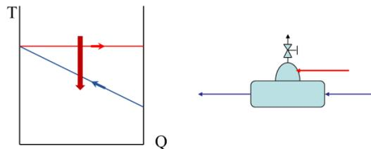
Figure 27: Schematic figure of deaerator and the heat transfer process
