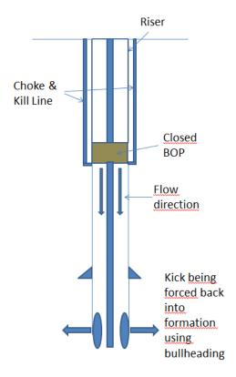
One well control method is based on pumping the kick back into the formation. This is called bullheading. In this case we will circulate mud down the choke and kill line simultaneously and it is important that the rate is large enough to overcome gas migration in the annulus such that we are able to force the kick downwards. In the following calculations we will assume that the density of the fluid is constant.
