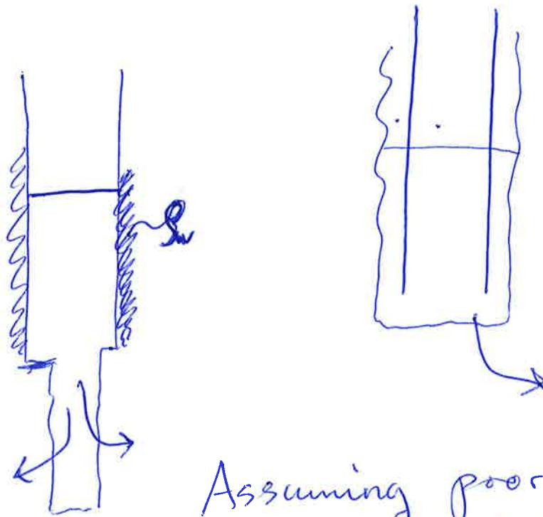
Assuming poor cement job  $\Rightarrow S_m$  outside casing
