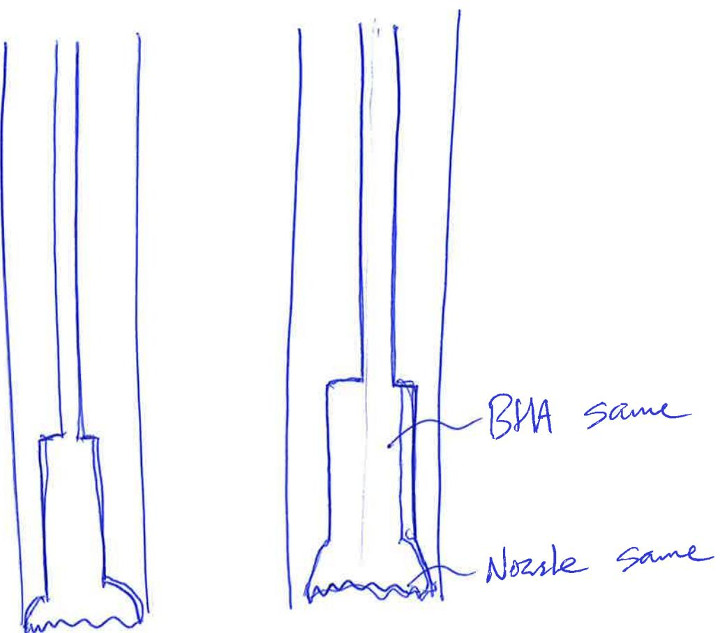
5"  $\Rightarrow$  ~~more flow~~ less parasitic pressure loss inside drillpipe
