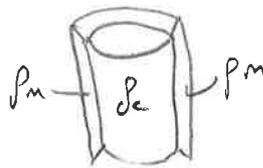
$$\begin{aligned} \Delta P_B &= P_i - P_o \\ &= 1550 \cdot 9,81 \cdot 3000 - 1180 \cdot 9,81 \cdot 3000 \\ &= \underline{\underline{108,9 \text{ bar}}} \quad \leftarrow (3\%) \end{aligned}$$
