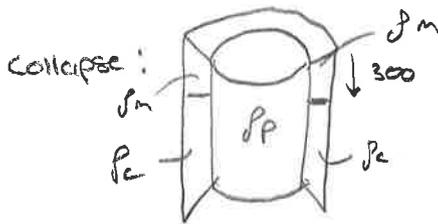
$$\begin{aligned} \Delta P_c &= P_o - P_i \\ &= [1550 \cdot 9,81 \cdot (3000 - 300) + 1180 \cdot 9,81 \cdot 300] \\ &\quad [1050 \cdot 9,81 \cdot 3000] \\ &= 445,3 - 309,0 \Rightarrow \underline{\underline{136,26 \text{ bar}}} \end{aligned}$$
