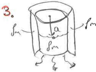
$$\begin{aligned} \Delta P_c &= P_o - P_i \\ &= 0,4 \cdot 3000 \cdot 1180 \cdot 9,81 - 0 \quad (2\%) \\ &= \underline{\underline{138,91 \text{ bar}}} \end{aligned}$$
