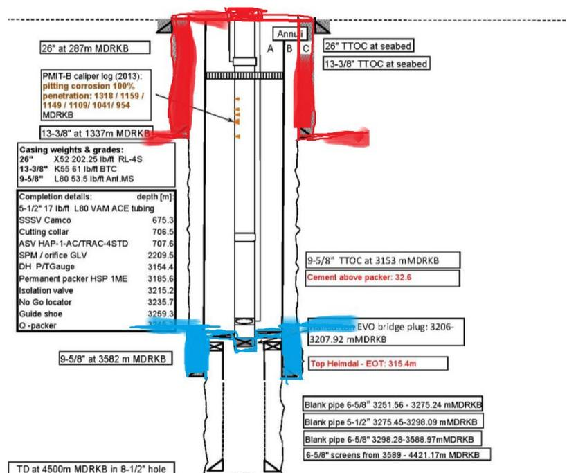
A.5: A well barrier diagram is created as an illustrative purpose so we can see all possible leak paths from the reservoir to its surrounding, and the WBD describes the status of a barrier element after a leak occurs.
