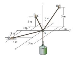
Force Vectors: We can express each of the forces on the free-body diagram shown in Fig. (a) in Cartesian vector form as
