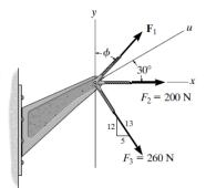
\*2–52. If the magnitude of the resultant force acting on the bracket is to be 450 N directed along the positive u axis, determine the magnitude of  $\mathbf{F}_1$  and its direction  $\phi$ .
