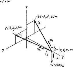
\*2-120. Determine the magnitude of the projected component of force  $\mathbf{F}_{AB}$  acting along the z axis.
