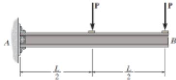
**Moment Area Theorem.** Since  $A$  is a fixed support,  $\theta_A = 0$ . Referring to the geometry of the elastic curve, Fig. *b*,
