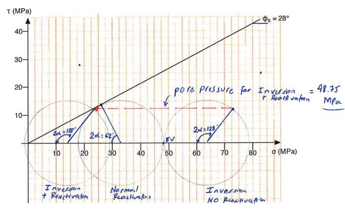
**a.** At a depth of 2 km, what is the differential stress  $(\sigma_1 - \sigma_3)$  for fault reactivation? Draw a Mohr circle for this case.
