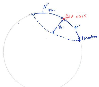
No strain on top of unit 1, therefore angle between fold axis and lineation is averywhere the same.
