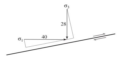
Using the graph paper below, show why this example is wrong. i.e. Construct the Mohr Circle diagram for this case, and estimate the actual normal and shear tractions acting on the fault plane.
