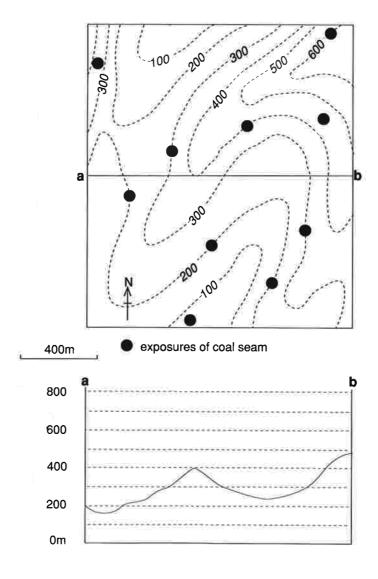
**a.** Construct structure contours of the contact every 100m (i.e. 100, 200, 300, 400, 500, and 600 m structure contours).
